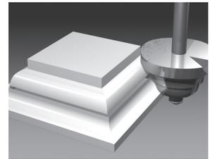
For Milling\Cutting\Engraving it is recommend to use a Single Flute\Tooth 'UP Cut Bit' (Left Hand Bit). The recommend cutting diameter ( $d$ ) is 4 mm; the Length of cut ( $l$ ) is 12 mm.
