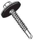
#12-14 x 1-1/4" HWH w/1-1/8" Oversize Bonded Washer (pre-drilling w/oversize holes required) Figure 15c
