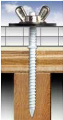
Fastener placement and spacing is first laid out on the wall, making sure to align fasteners with framing members behind the outer wall. Fasteners should be spaced no further than 12" apart around the perimeter of the panel (see illustration at right). Fasteners placed in corners should be a minimum of 2" to a maximum of 6" from each edge of the corner of the panel.
